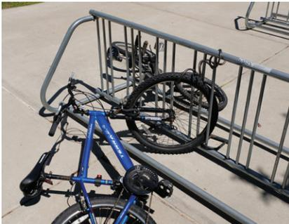
Rack does not provide 2 points of support or place to lock to frame (Photo: MIG/SvR)
